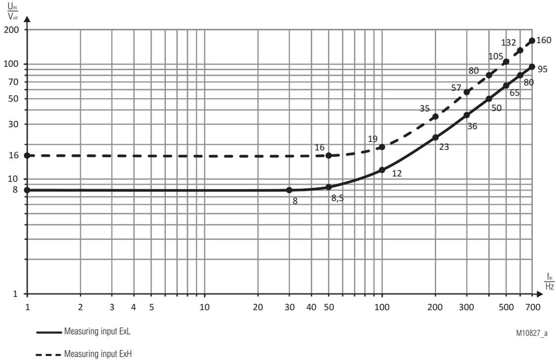
Min. voltage at measuring input for variant /0\_\_
