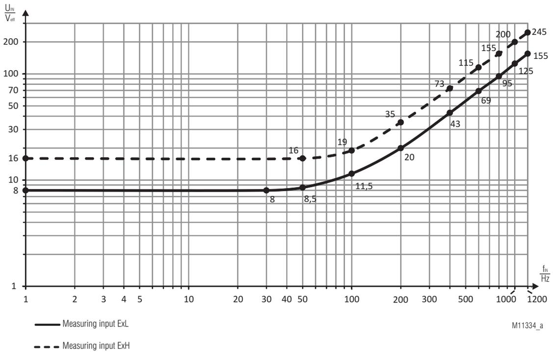
Min. voltage at measuring input for variant /1\_\_
