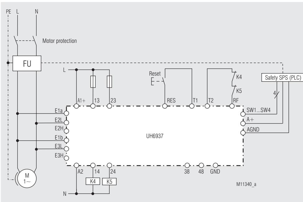
Inverter monitoring function, single-phase with variant UH6937/\_ \_1;
